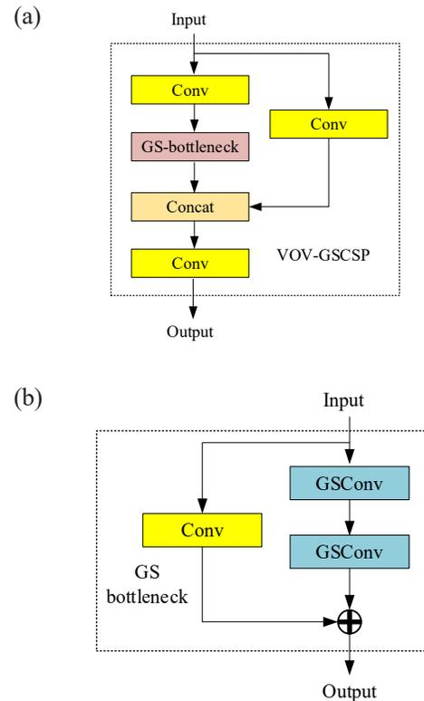
Figure 2. (a) VoVGSCSP layer; (b) GS-bottleneck layer
